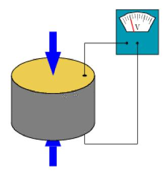
If mechanical pressure is applied to the opposite faces of the crystal , potential difference is developed ,which would be proportional to the pressure applied .
